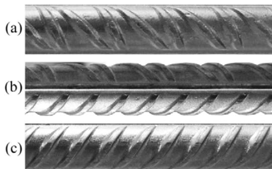
Fig. 1 Overview of the steel rebar rib patterns
