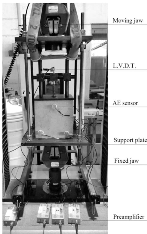
Fig. 4 Experimental setup
