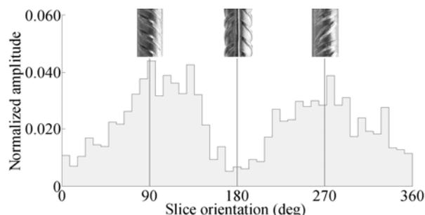
Fig. 13 Distribution of damage intensity around the rebar perimeter
