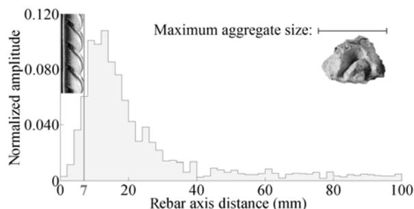
Fig. 12 Damage intensity as a function of the rebar axis distance
