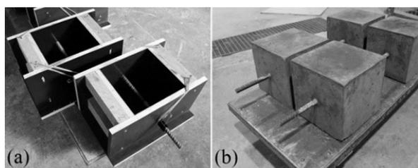
Fig. 2 (a) Formworks, (b) Hardened pull-out specimens
