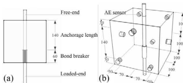
Fig. 3 (a) Interface design, (b) AE sensor distribution
