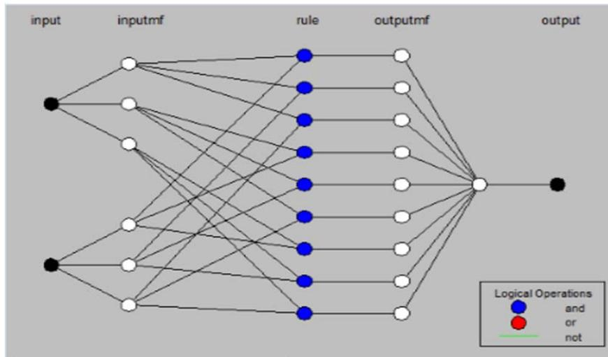
Fig. 2 A typical ANFIS model structure for rain attenuation values at different rain rates and frequencies.
