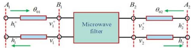
Fig. 3 S-parameter matrix of two port network
