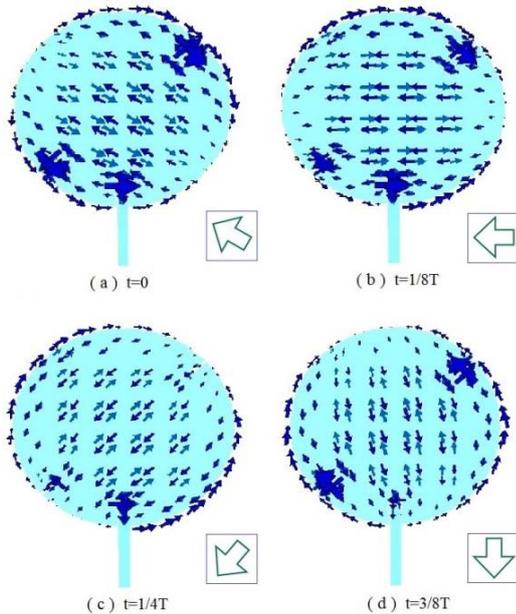
Fig. 13 The current distribution on the surface of the middle ring with radius of  $R_2$
