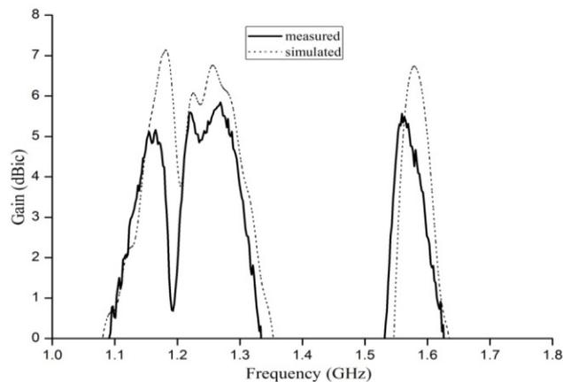
Fig. 11 Simulated and measured gain of the antenna
