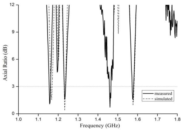
Fig. 7 Simulated and the measured axial-ratio of the antenna
