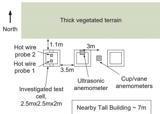
Fig. 1 Top view of setup and critical dimensions.
