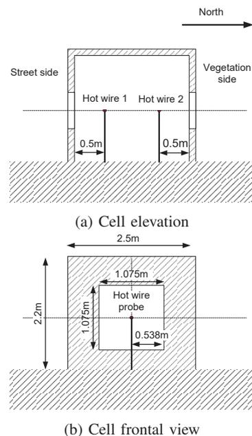
Fig. 2 Cell dimensions and hot wire positions
