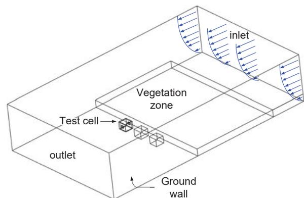
Fig. 4 Geometry of the model with boundary conditions shown. Side walls and top 'lid' are prescribed as symmetry boundary conditions
