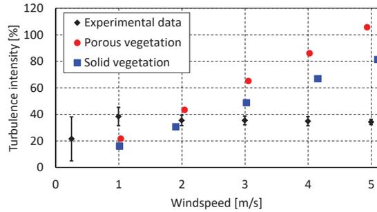
Fig. 12 Turbulence intensity against wind speed at the cup anemometer location
