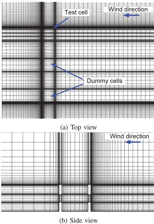
Fig. 6 Mesh details close to the test cell
