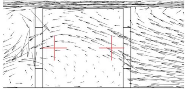
Fig. 3 Velocity vectors indicating flow directions. Left cross-hair indicates hot wire 2 while right cross-hair indicates hot wire 1. The case shown here is for solid vegetation at a 5m/s reference wind speed
