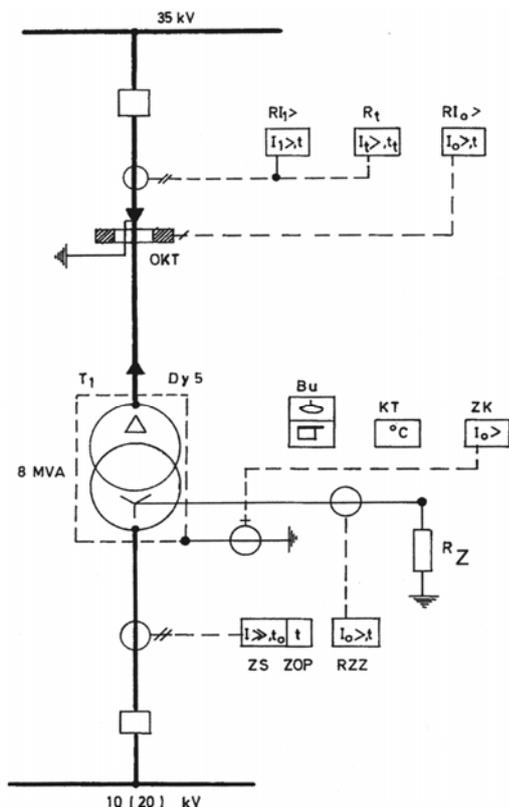
Fig. 2 Transformer protection in TS 35/10.5 kV/kV
