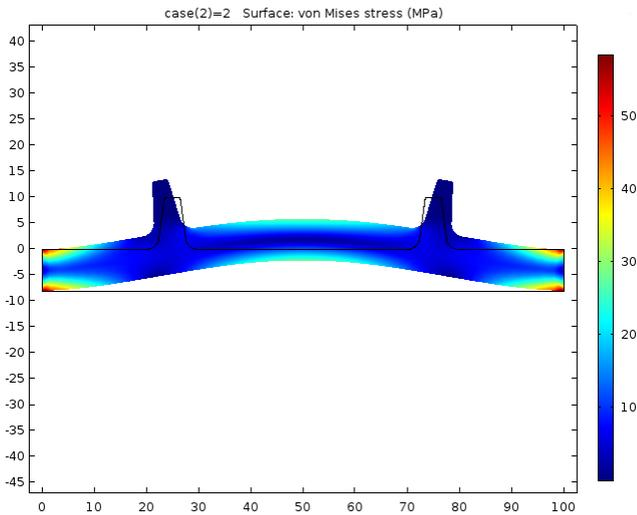
Fig. 5 Stresses on disc geometries (with ribs)
