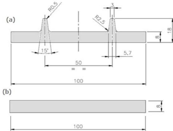
Fig. 2 (a) Disc with ribs / (b) flat plate
