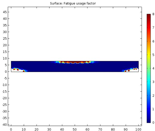
Fig. 8 Fatigue usage factor (flat)
