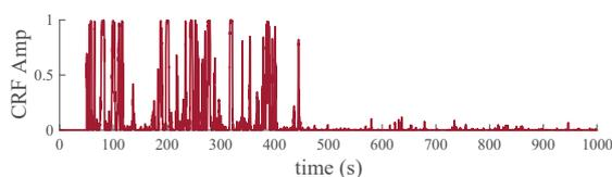
Fig. 7 P-wave detector output directly from STA/LTA data
