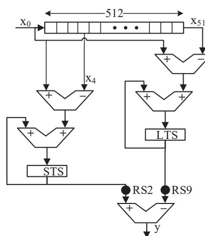
Fig. 4 Architecture of the STA/LTA block
