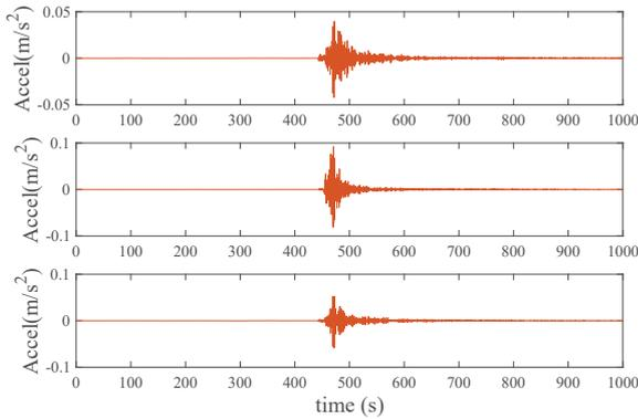
Fig. 6 STA/LTA block output for 3-axis seismic data
