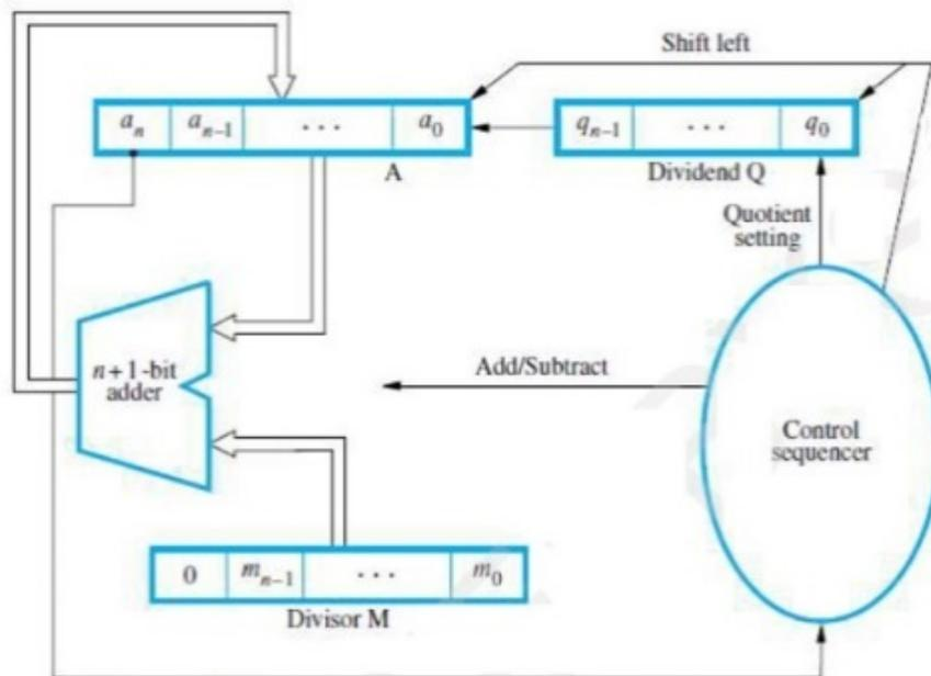
Fig. 1 Block diagram for binary division [3]
