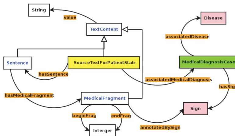
Fig. 4 Overall data structure to diagnostics recommendation system
