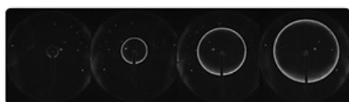
Fig. 2 Spherical flame propagation, for 0.5 MPa,  $\Omega=1.0$ ,  $X(\text{H}_2\text{O})=0.65$ ,  $T_0=473$  K,  $\Phi=1$ , in which the flame is propagated normally
