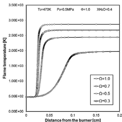
Fig. 8 Flame temperature profiles for stoichiometry methane/oxygen enriched flames with  $\text{H}_2\text{O}$  dilution. ( $\Omega$  from 0.3 to 1.0,  $T_0=473$  K,  $P_0=0.5$  MPa,  $X(\text{H}_2\text{O})=0.4$ )
