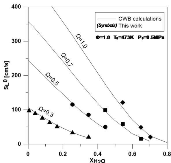
Fig. 11 Comparison between experimental (our results: symbols) and calculated (with CWB and GRIMEch3.0, solid lines) fundamental laminar burning velocities,  $S_L^0$ , in  $cm.s^{-1}$ , as a function of  $H_2O$  dilution,  $X(H_2O)$ , for a pressure  $P_0=0.5$  MPa,  $\phi=1$  and  $T_0=473$  K
