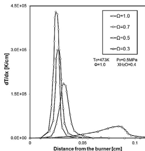
Fig. 9 Temperature gradients for stoichiometry methane/oxygen enriched flames with  $\text{H}_2\text{O}$  dilution. ( $\Omega$  from 0.3 to 1.0,  $T_0=473$  K,  $P_0=0.5$  MPa,  $X(\text{H}_2\text{O})=0.4$ )
