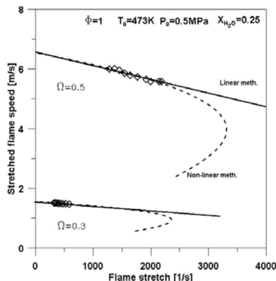
Fig. 4 Stretched flame speed in m/s as a function of flame stretch (in  $\text{s}^{-1}$ ) for  $\Omega=0.3$  and  $0.5$ ,  $\Omega=1$ ,  $X\text{H}_2\text{O}=0.25$  and  $P=0.5$  MPa. Symbol: experimental velocity as a function of flame stretch, dashed line: nonlinear methodology, solid line: linear extrapolation methodology
