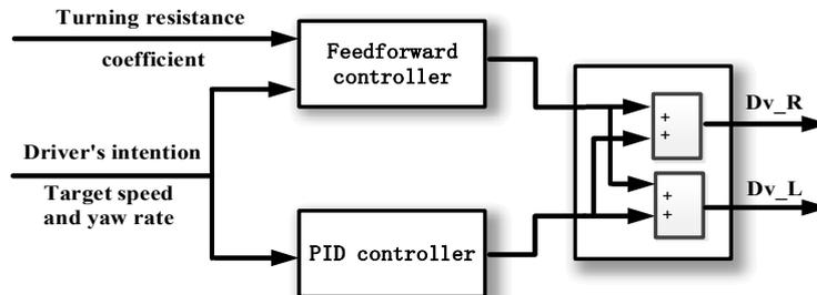
Fig. 9 Feedforward Control
