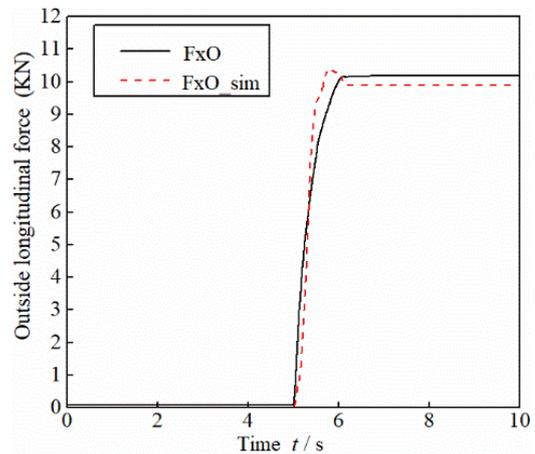
Fig. 5 Outside wheel longitudinal force
