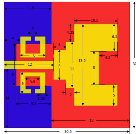
Fig. 1 Geometry of the proposed antenna structure
