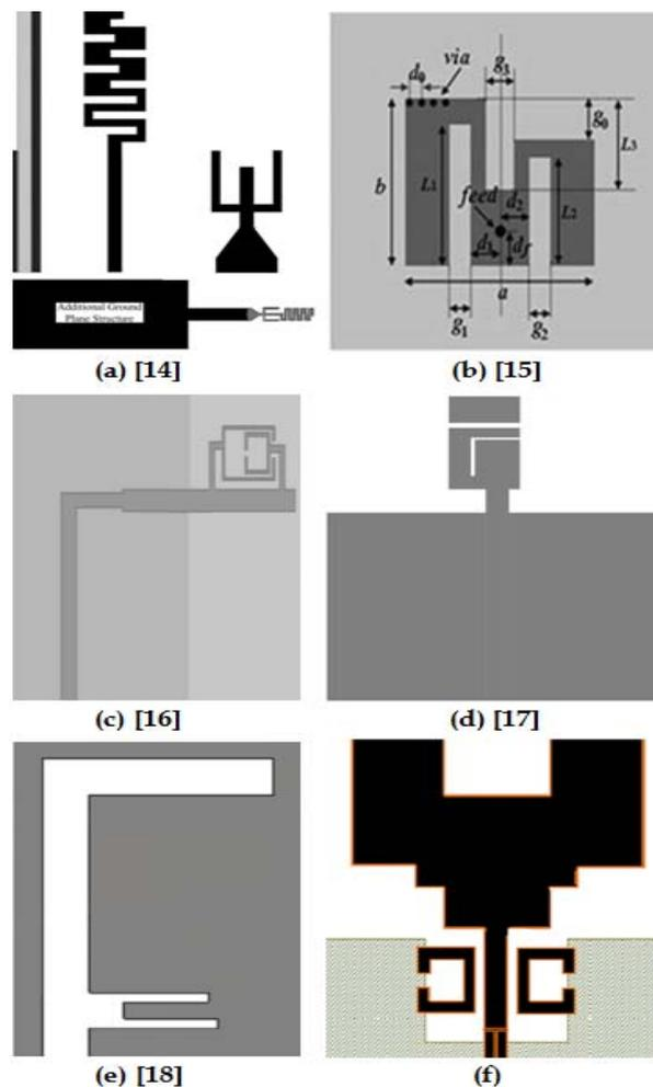
Fig. 10 Comparison of size of the proposed antenna with other references, (a)  $60 \times 40 \text{ mm}^2$ , (b)  $64 \times 62 \text{ mm}^2$ , (c)  $60 \times 90 \text{ mm}^2$ , (d)  $33 \times 90 \text{ mm}^2$ , (e)  $40 \times 45 \text{ mm}^2$ , and (f) the proposed miniaturized structure  $30 \times 30.5 \text{ mm}^2$
