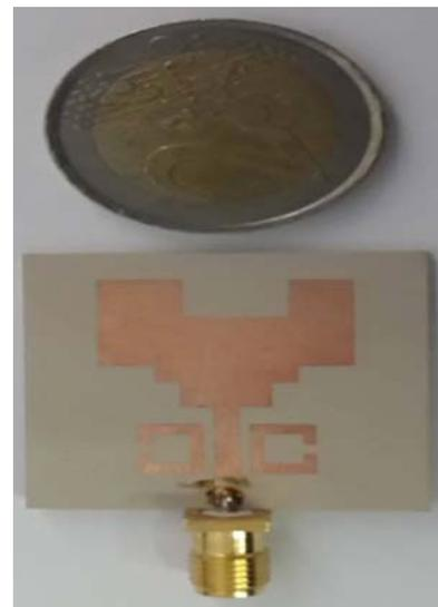
Fig. 7 Fabricated prototype of the proposed antenna
