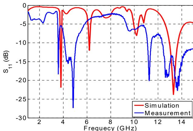
Fig. 9 Simulated and measured reflection coefficient of proposed tri-band antenna
