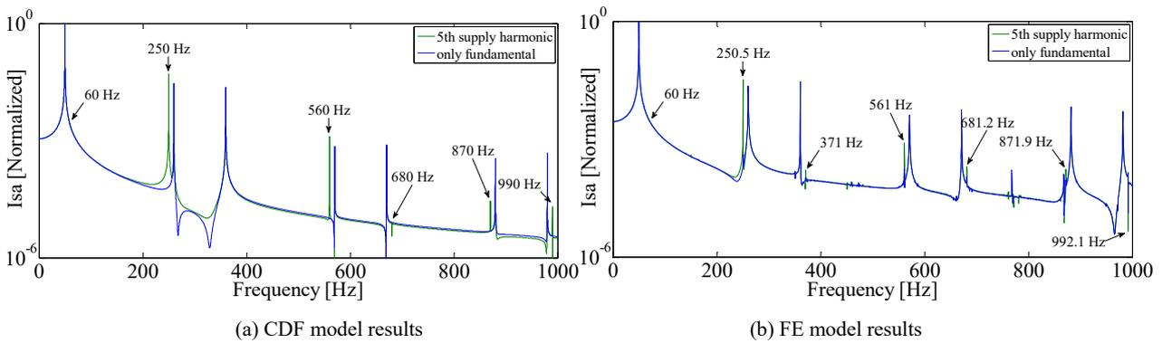
A-phase stator current spectrum from the CDF and FE models for the fundamental and 5<sup>th</sup> order supply harmonics
