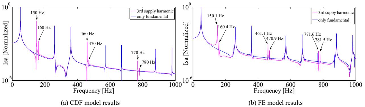
Fig. 4 A-phase stator current spectrum from the CDF and FE models for the fundamental and 3<sup>rd</sup> order supply harmonics
