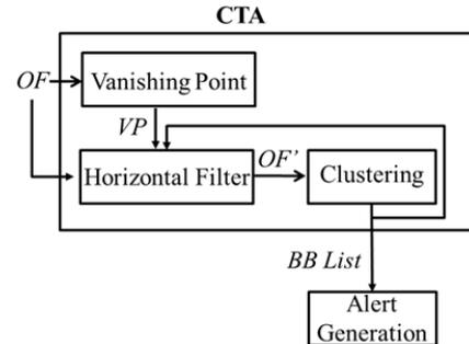
Fig. 2 Block based schema of the CTA algorithm
