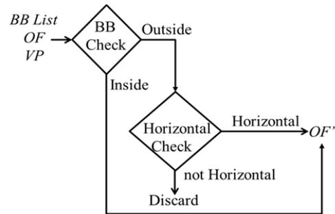
Fig. 4 Block based schema of Horizontal Filter step
