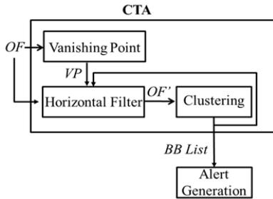
Fig. 3 Block based schema of VP step
