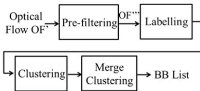
Fig. 7 Block based schema of Clustering step
