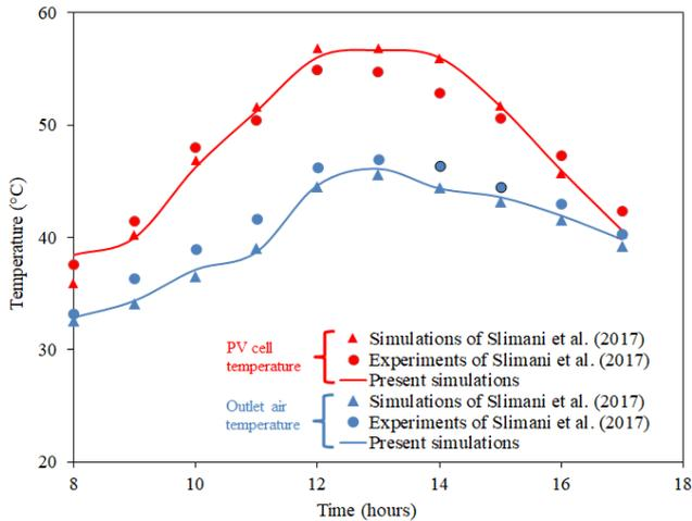
Fig. 3 Temporal variations of the PV cell and outlet air temperatures. Comparisons between the present results and the experiments and simulations of Slimani et al. [26] for  $w=1 \text{ m.s}^{-1}$ .  $V_{in}$  and  $G$  vary with time
