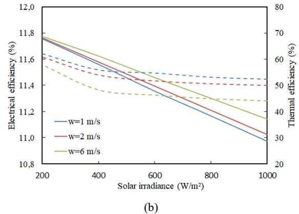
Fig. 8 Variation of (a) the PV cell (solid lines) and outlet air (dashed lines) temperatures and (b) the electrical (solid lines) and thermal (dashed lines) efficiencies with the solar irradiance. Results obtained for three wind speeds and  $V_{in} = 2 \text{ m}\cdot\text{s}^{-1}$ ,  $H=20 \text{ mm}$  and five ribs
