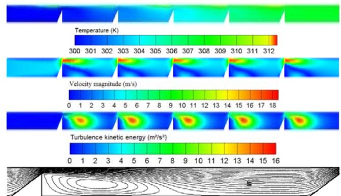
Fig. 4 Maps of temperature (K), velocity magnitude (m/s) and turbulence kinetic energy ( $\text{m}^2/\text{s}^2$ ). Zoom between the second and third ribs highlighting the streamline patterns. Results obtained for 5 ribs with  $H=20 \text{ mm}$ ,  $w=1 \text{ m.s}^{-1}$  and  $V_{in}=3.5 \text{ m.s}^{-1}$
