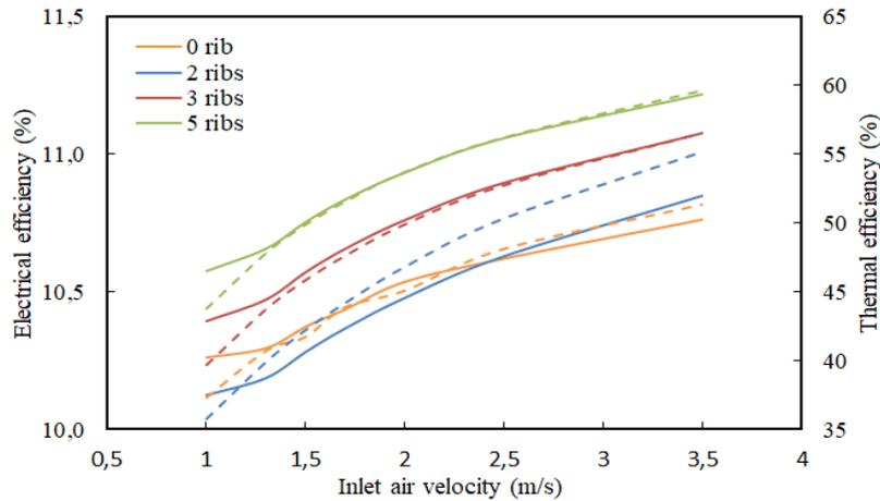
Fig. 7 Variations of the electrical (solid lines) and thermal (dashed lines) efficiencies as a function of the inlet air velocity for four rib configurations ( $w=1 \text{ m}\cdot\text{s}^{-1}$ ,  $H=20 \text{ mm}$ )
