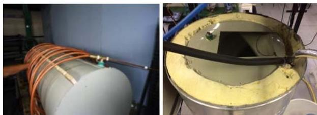
Fig. 2 Gas cooler assembly
