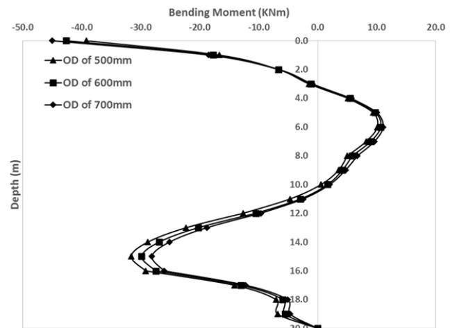
Fig. 15 Effects of supporting system rigidity on rear pile row bending moment
