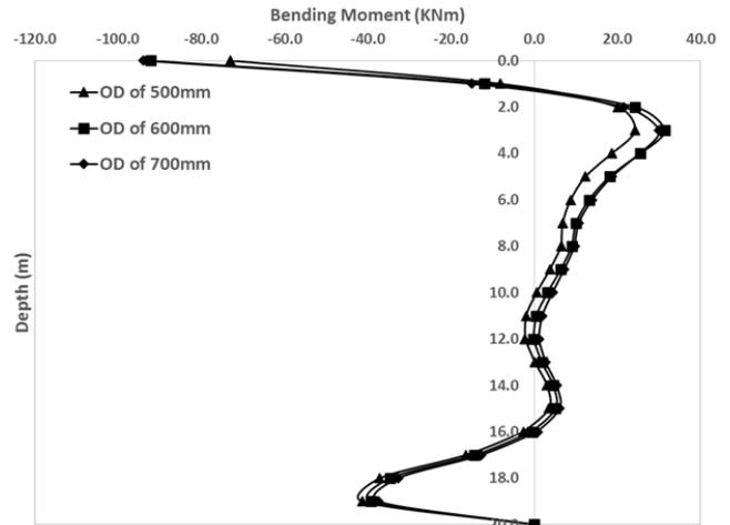
Fig. 14 Effects of supporting system rigidity on front pile row bending moment
