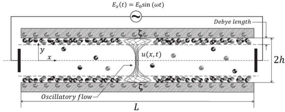
Fig. 1 Schematic model for an oscillatory electroosmotic flow moved by an externally electrical field defined by  $E_x(t) = E_0 \sin \omega t$ .  $E_0$  and  $\omega$  are the steady electric field and the angular frequency, respectively
