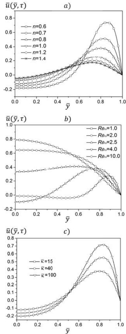
Fig. 3 Dimensionless velocity distribution  $\bar{u}(\bar{y}, \tau)$  vs  $\bar{y}$ , for various values of angular Reynolds number  $Re_\omega$ , dimensionless debye length  $\bar{\kappa}$  and the flow behavior index  $n$  at  $\lambda = 2$  and  $\tau = 1$ . (a)  $Re_\omega = 5$  and  $\bar{\kappa} = 15$ . (b)  $\bar{\kappa} = 15$  and  $n = 0.8$ . (c)  $n = 0.8$  and  $Re_\omega = 5$
