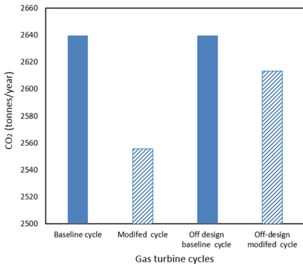
Fig. 5 Effect of improving the power turbine performance on the annual CO<sub>2</sub> emissions of the cycle, at design and off-design
