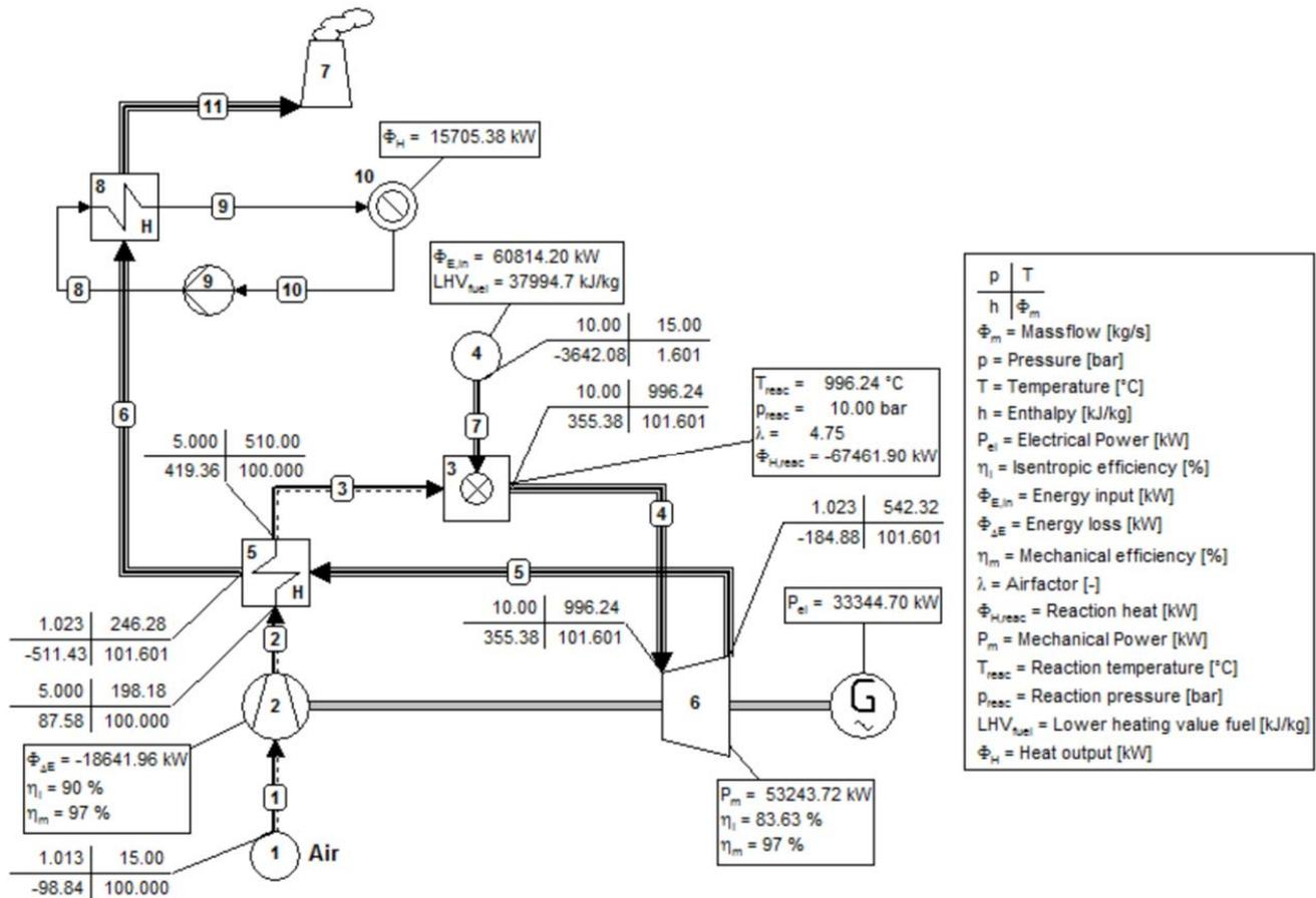
Fig. 1 Gas turbine cycle with regeneration and cogeneration processes using the optimized casing modelled with Cycle-Tempo
