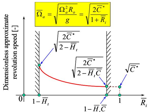
Fig. 9 Variation of the dimensionless approximate revolution speed of the DCGMG versus the dimensionless radius of the inner rail
