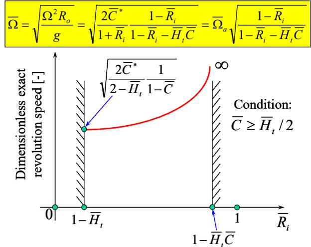
Fig. 11 Variation of the dimensionless exact revolution speed of the DCGMG versus the dimensionless radius of the inner rail, obtained under the condition:  $\bar{C} \geq \bar{H}_i / 2$
