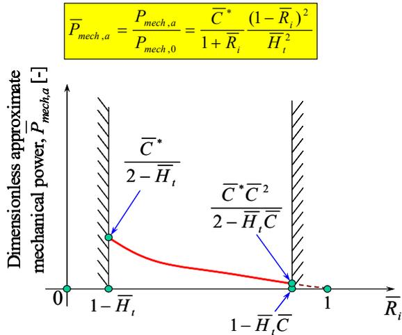
Fig. 19 Variation of the dimensionless approximate mechanical power inputted at the shaft of the motor-generator versus the dimensionless radius of the inner rail
