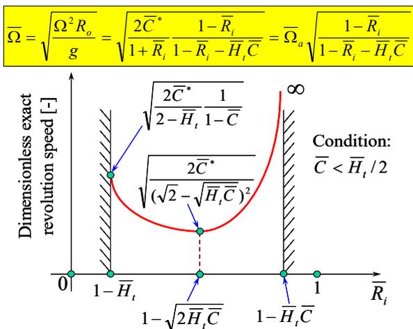
Fig. 10 Variation of the dimensionless exact revolution speed of the DCGMG versus the dimensionless radius of the inner rail, obtained under the condition:  $\bar{C} < \bar{H}_i / 2$
