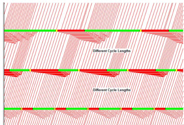
Fig. 9 Traffic Progression for Prince Shaker Bin Zaid under the Existing Conditions
