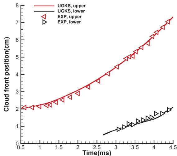
Fig. 4 Cloud upper and lower front trajectories from 2 cm bed of 1.5mm diameter glass spheres subject to Mach 1.3 shock in air ( $C_d = 12, C_{af} = 20$ )
