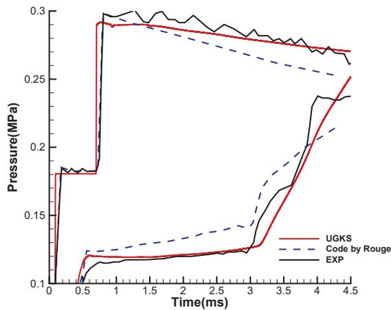
Fig. 3 Pressure signals upstream and downstream of the cloud; transducer location 11cm below and 4.3 mm above the support, 2 cm bed of 1.5mm diameter glass spheres subject to Mach 1.3 shock in air ( $C_d = 12, C_{af} = 20$ )
