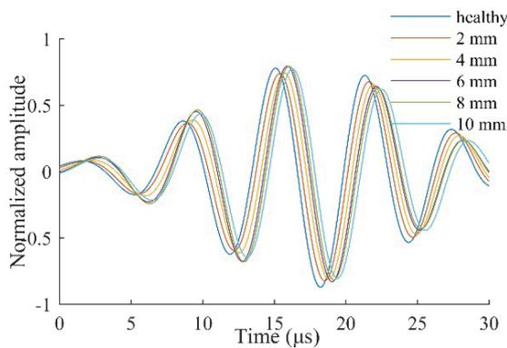
Fig. 4 Comparison of time window for healthy and different delamination sizes
