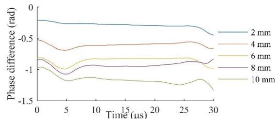
Fig. 6 Phase differences for different damage cases
