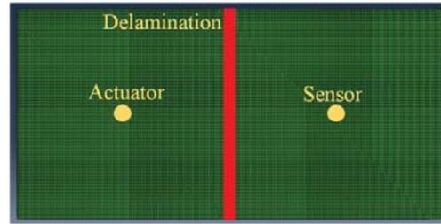
Fig. 1 Finite element model of composite plate
