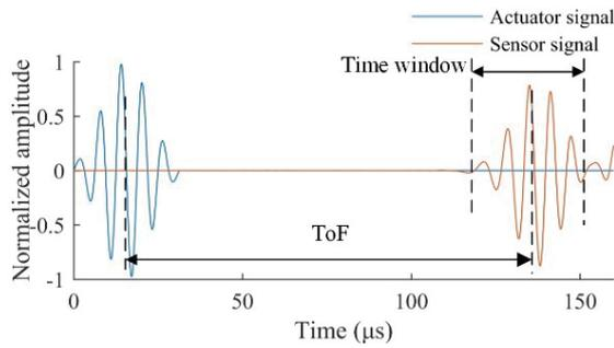
Fig. 3 Illustration of the ToF and time window
