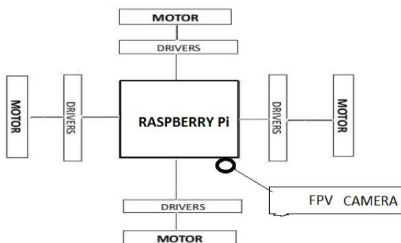
Fig. 7 Block diagram of quadcopter
