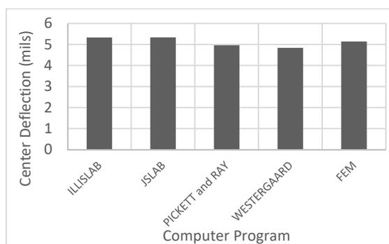
Fig. 1 Deflection comparison under interior load
