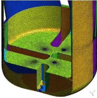
Fig. 3 Tetrahedral Mesh - Cut plane view
