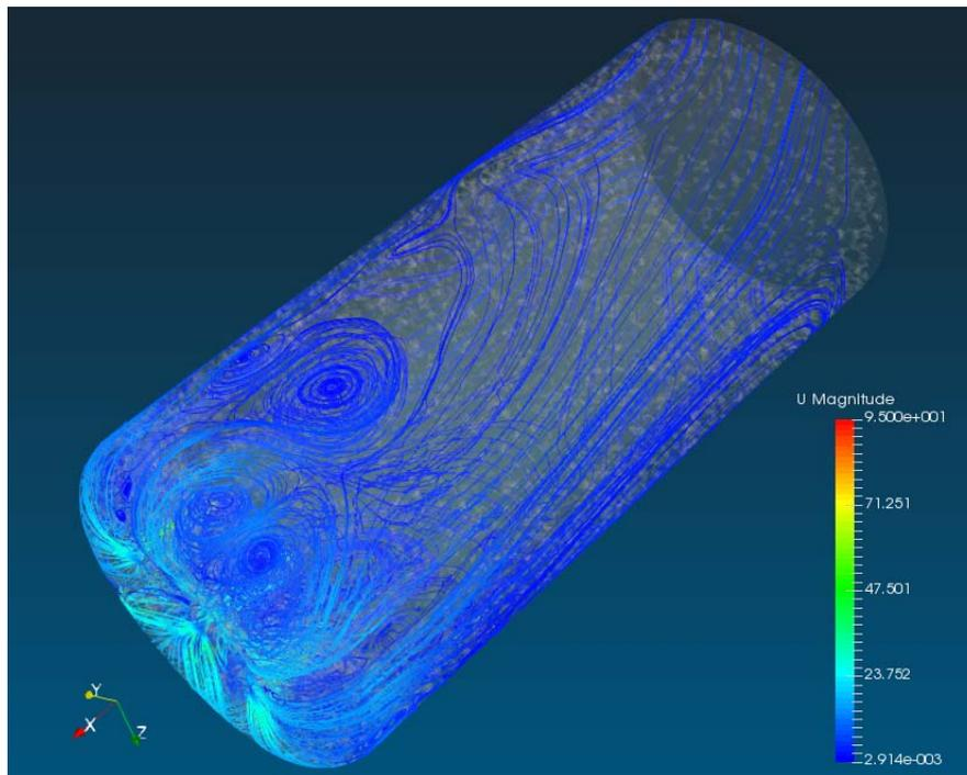
Fig. 5 (a) streamlines -Vaneless annulus
