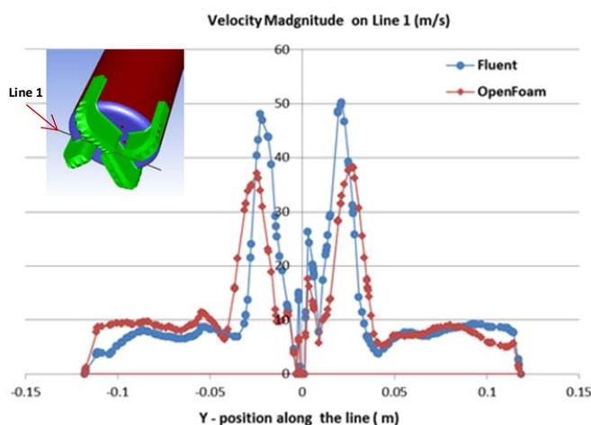
Fig. 7 Velocity magnitude comparisons on post-processing line OpenFOAM vs. ANSYS Fluent
