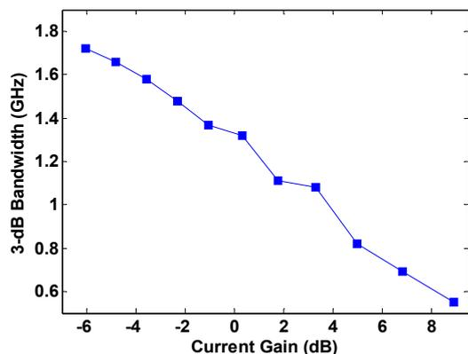
Fig. 6 The 3-dB bandwidth of proposed circuit versus current gain
