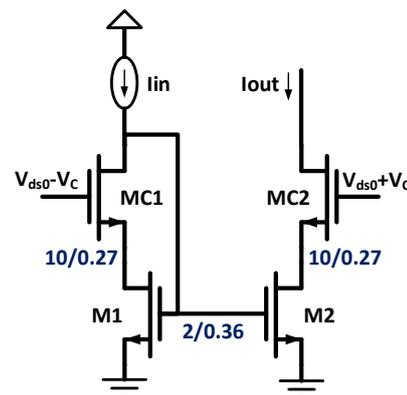
Fig. 1 Proposed high speed low power adjustable gain current mirror
