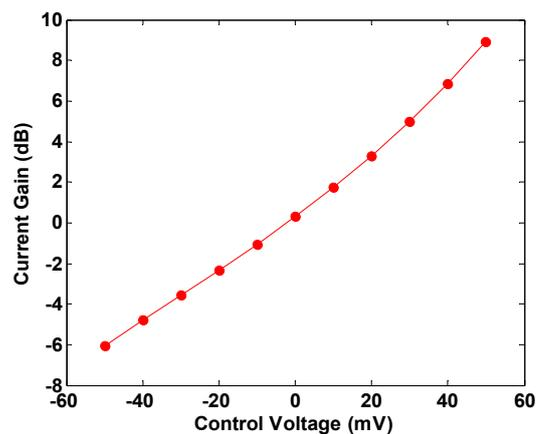
Fig. 5 The current gain versus control voltage
