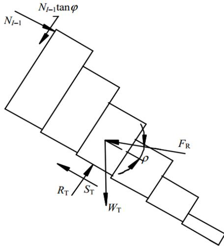
Fig. 5 Mechanical model of sliding front edge
