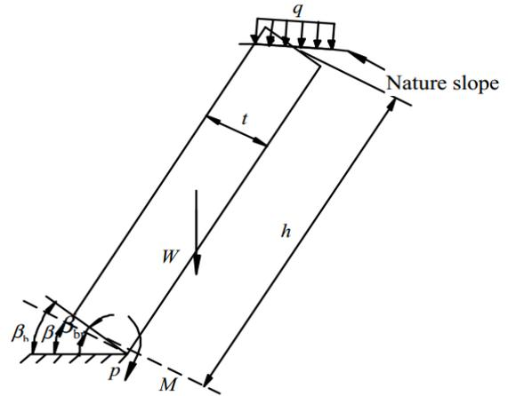
Fig. 2 Stability of a single rock block subjected to crest load
