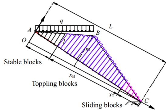
Fig. 4 Schematic of slope failure mode
