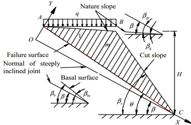
Fig. 1 Geometric geometry model of the toppling failure
