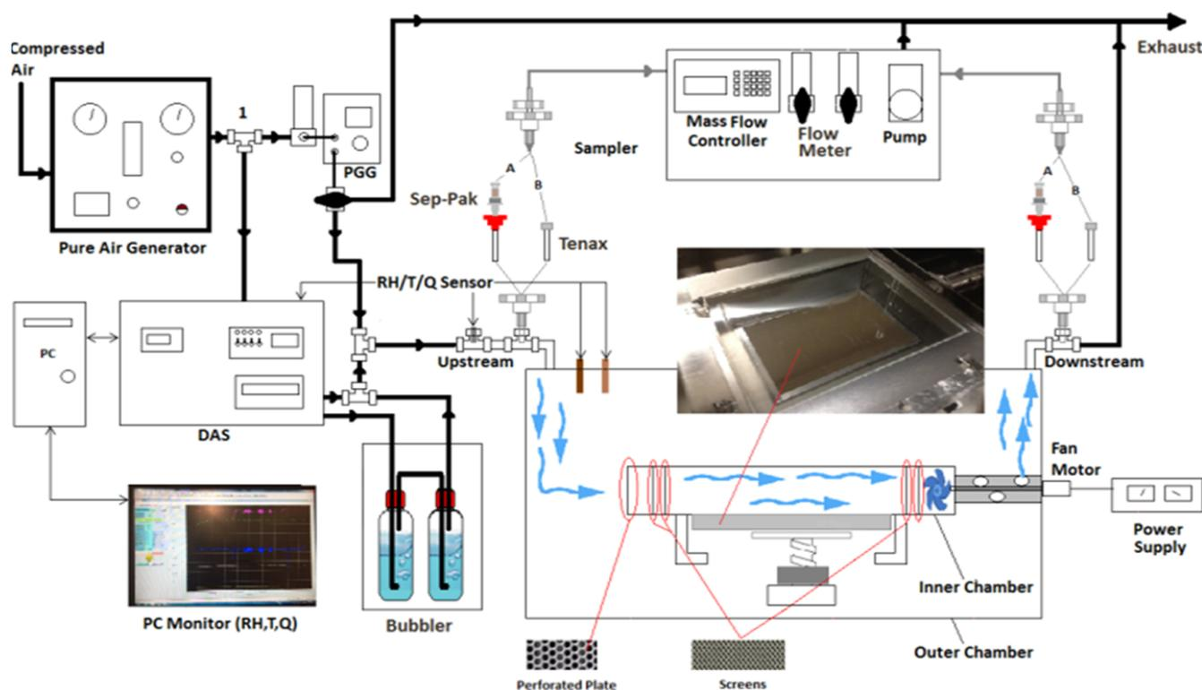
Fig. 1 Schematic diagram of the IPPT test chamber
