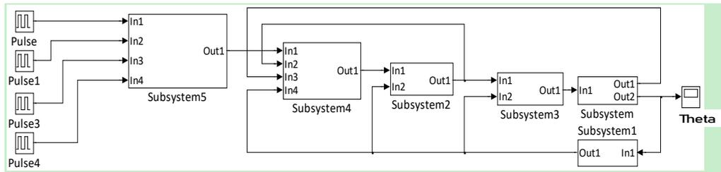
Fig. 4 MATLAB/Simulink model of the stepping motor
