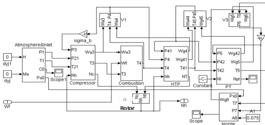
Fig. 5 Component level model of the turboshaft engine
