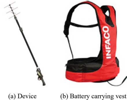
Fig. 6 Commercially available portable solution for blossom thinning [23]
