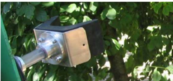
Fig. 1 Limb shaker without a mechanical coupling to the branches [6]
