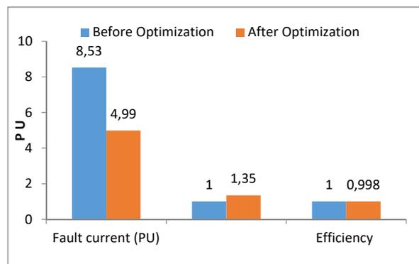
Fig. 7 Fault current reduction optimization
