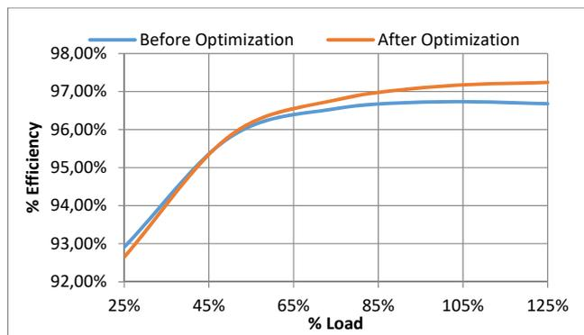
Fig. 6 Efficiency comparison in “maximum efficiency optimization”
