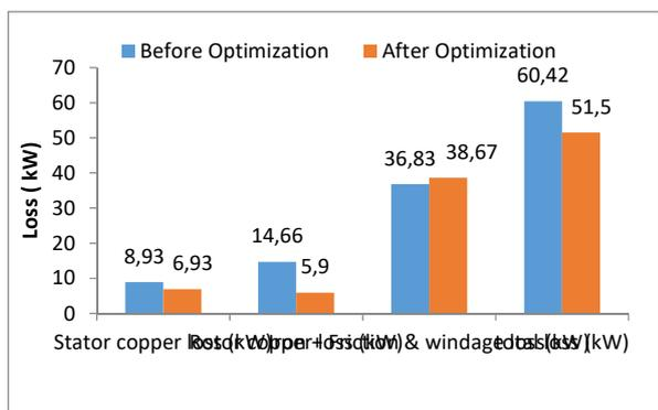
Fig. 5 Loss comparison in “maximum efficiency optimization”
