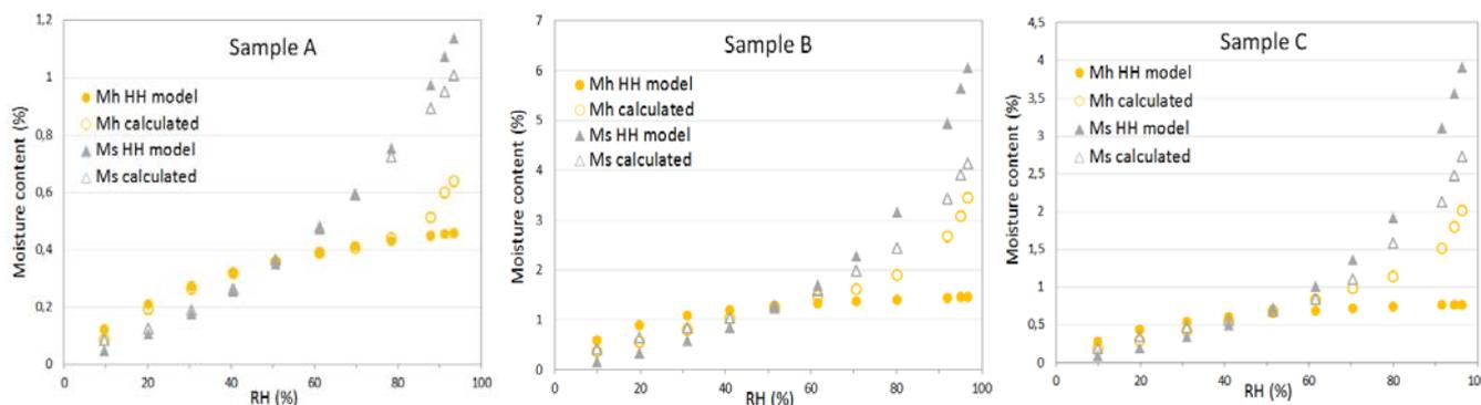
Fig. 6 HH model (M<sub>h</sub> monolayer, M<sub>s</sub> polylayer) and HH model calculated
