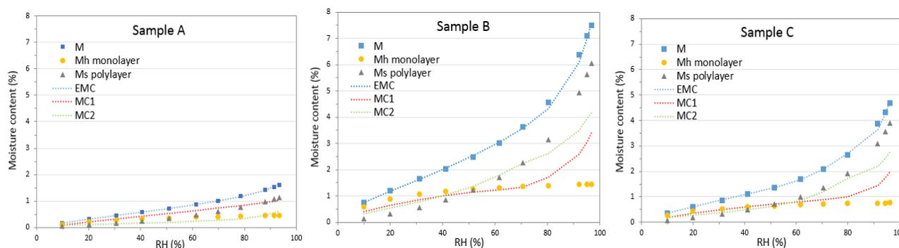
Fig. 5 HH model (M, Mh monolayer, Ms polylayer) and PEK model (EMC, MC<sub>1</sub> and MC<sub>2</sub>)
