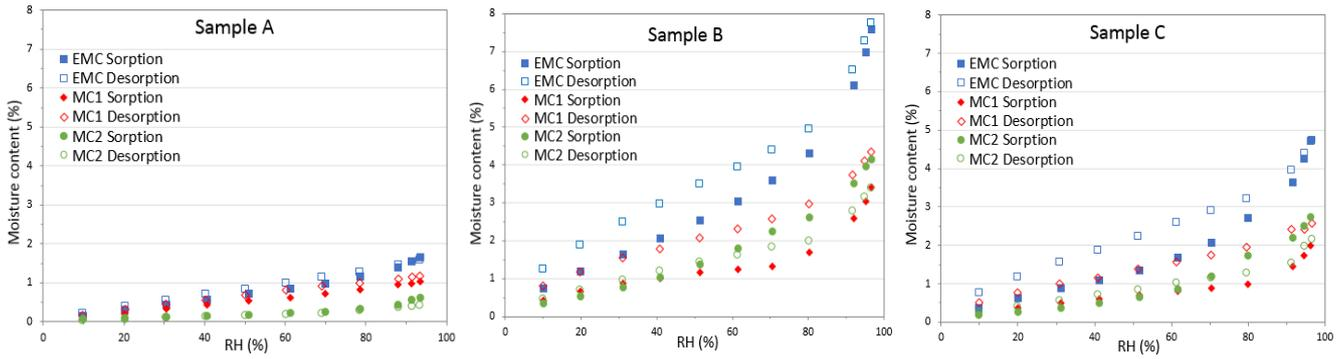
Fig. 1 Moisture content for EMC, fast (MC<sub>1</sub>) and slow (MC<sub>2</sub>) sorption and desorption processes
