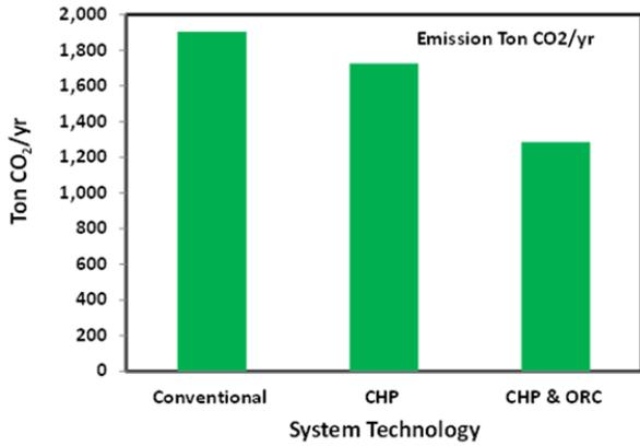
Fig. 62 CO<sub>2</sub> emission from different technologies
