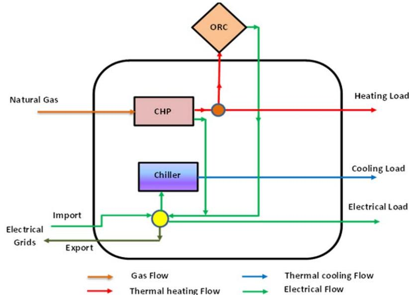
Fig. 2 Schematic of energy modeling and technology details at each hub for case 3 (CHP & ORC system)
