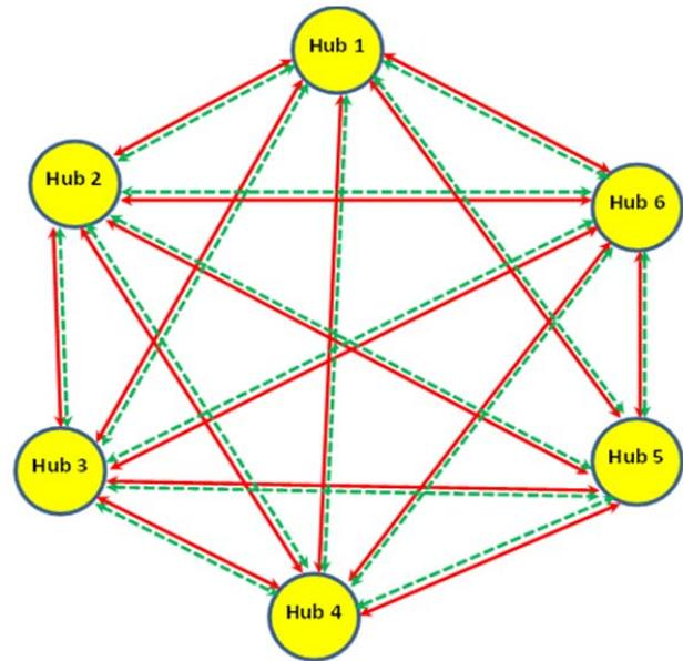
Fig. 1 Energy transfer between hubs and grids (red lines are for thermal and green dot lines are for electrical)
