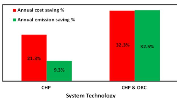
Fig. 84 Overall cost and CO<sub>2</sub> emission saving compared to the conventional system
