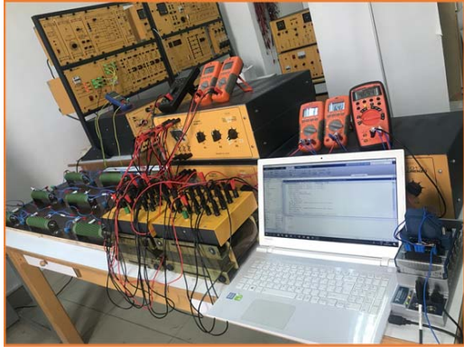
Fig. 3 Laboratory model of AQSA electric power system
