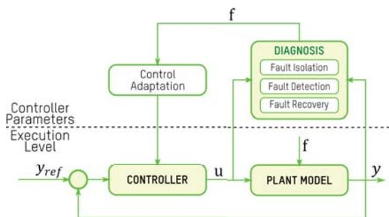
Fig. 2 Architecture for Active Fault-Tolerant Control Systems
