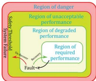
Fig. 1 Regions of performance: required and degraded
