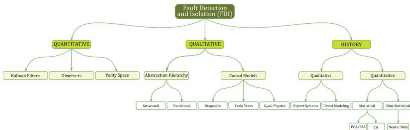
Fig. 4 Fault Detection and Identification (FDI) methodologies
