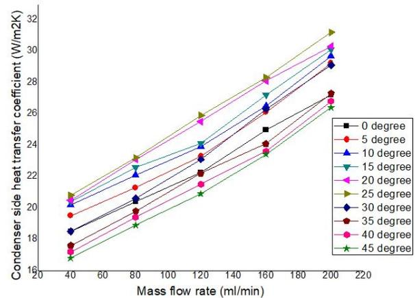
Fig. 6 Comparisons of condenser heat transfer coefficient with mass flow rate at different angle of inclination
