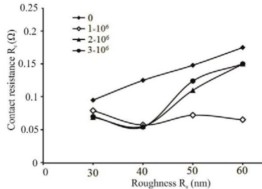
Fig. 5 Dependence of the contact resistance on roughness
