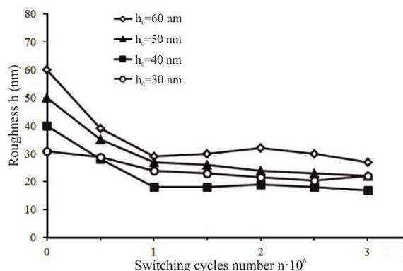
Fig. 6 Dynamics of the roughness change during switching
