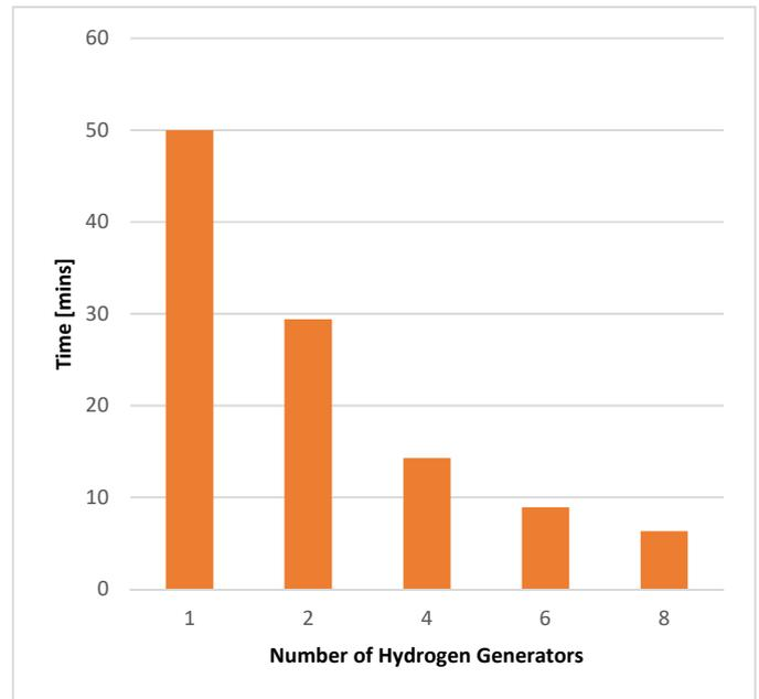
Fig. 6 Time required to refill a 50 liter gas cylinder
