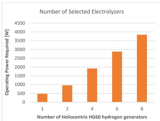
Fig. 5 Required number of Heliocentris HG60 hydrogen generator
