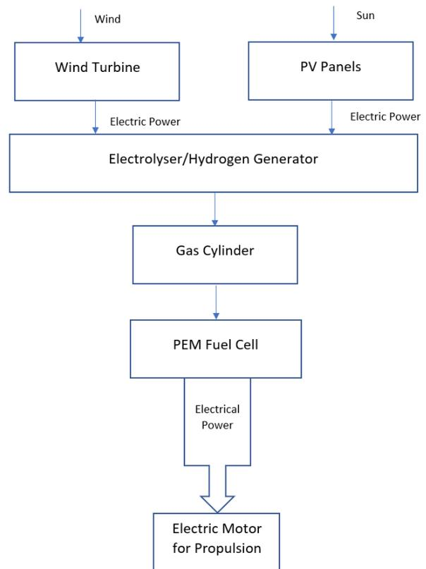
Fig. 1 Schematic of the HRES for electric boats
