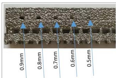
Fig. 4 Small fabricated holes
