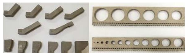
Fig. 12 Fabricated overhang test specimens by EBM
