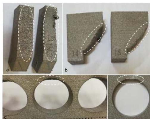
Fig. 13 Overhang structures distortions
