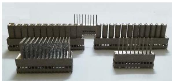
Fig. 3 Fabricated test specimens by EBM
