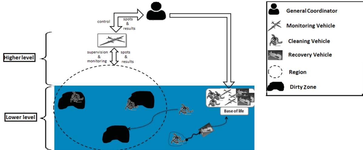
Fig. 1 Deployment of our centralized system based on a Coordinator, UAVs, USVs and Recovery vehicles
