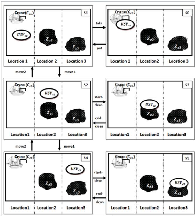
Fig. 4 A state-transition system for USV-Cleaning domain
