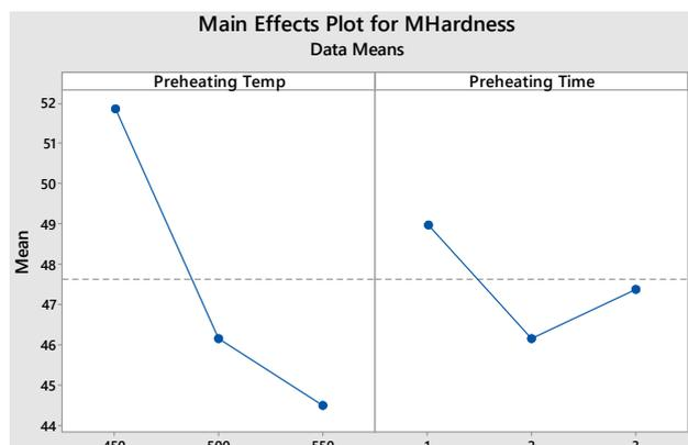
Fig. 5 Main effect plot for microhardness
