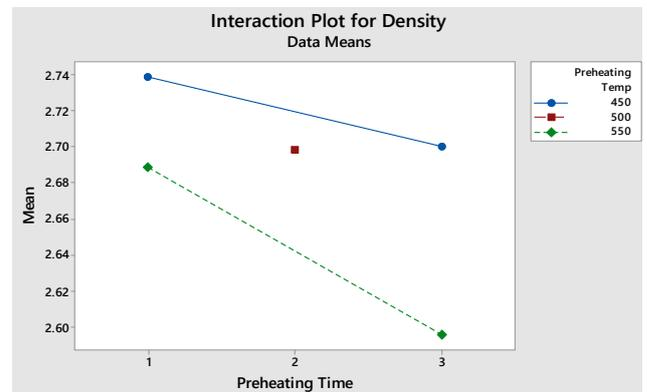
Fig. 8 Interaction plot for density
