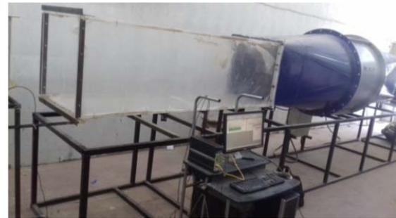
Fig. 2 Wind tunnel used for flow generation
