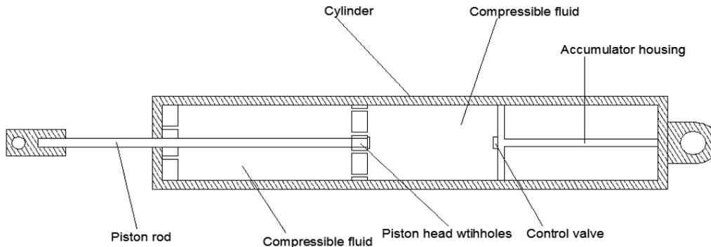
Fig. 1 Typical viscous damper
