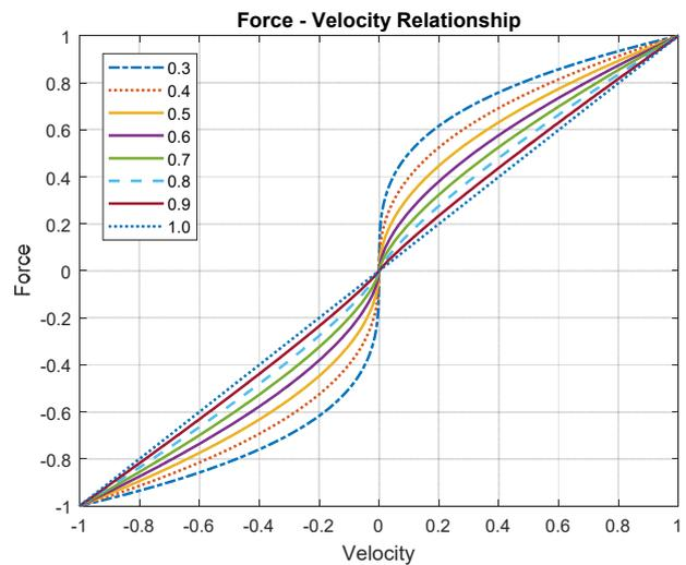
Fig. 2 Force-velocity relationship for various values of  $\alpha$
