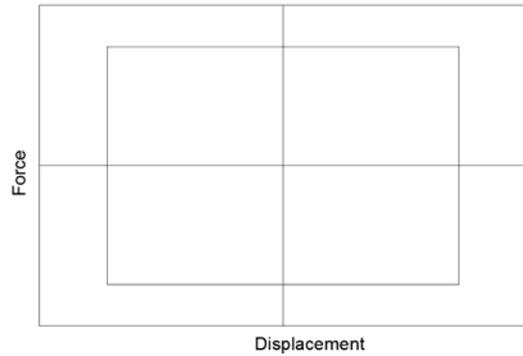
Fig. 6 Idealized force-displacement relationship of friction damper
