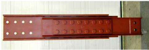
Fig. 4 Friction Damper
