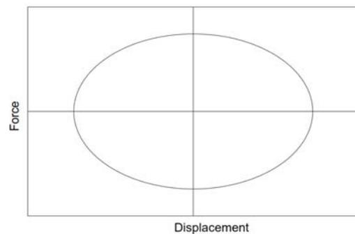
Fig. 3 Idealized force displacement relationship of viscous damper
