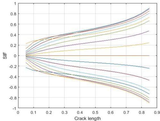
Fig. 5 Variation of  $K_{II}$  w.r.t crack length for different  $\alpha$
