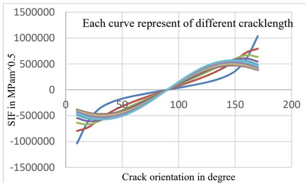
Fig. 10 Variation of  $K_{II}$  w.r.t crack orientation ( $\alpha$ )
