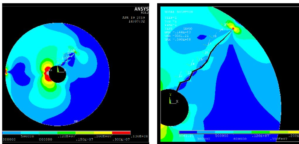
Fig. 13 Crack propagation using crack-kinking concept (a) at early stage, (b) just before physical separation
