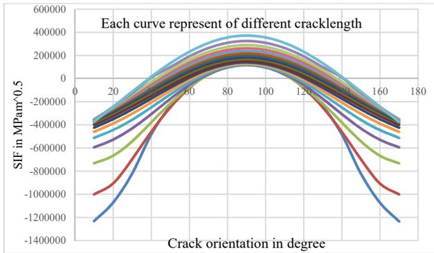
Fig. 9 Variation of  $K_I$  w.r.t crack orientation ( $\alpha$ )
