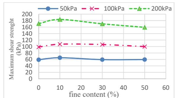
Fig. 5 Maximum shear strength versus the fine content in three vertical stress of 50, 100, and 200 kPa
