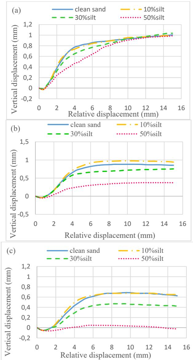
Fig. 6 Vertical displacement versus relative displacement curves of silty sand samples under three vertical stress; (a) 50 kPa; (b) 100 kPa (c) 200 kPa
