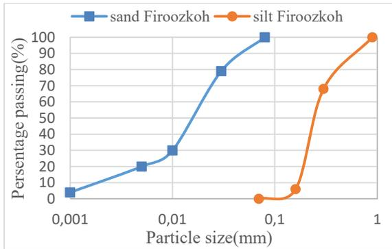
Fig. 2 Particle size distribution curves of tested materials
