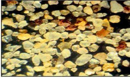
Fig. 1 Microscopic image of tested Firoozkoo sand
