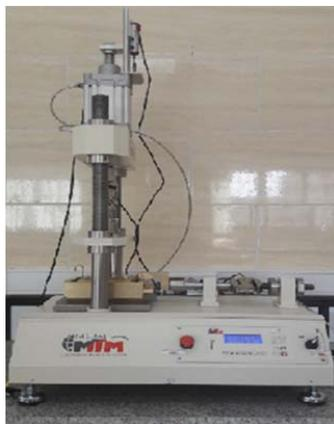
Fig. 3 Digital direct shear apparatus in IKIU lab
