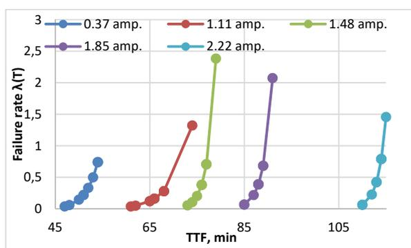
Fig. 8 Failure rate for the different stress levels
