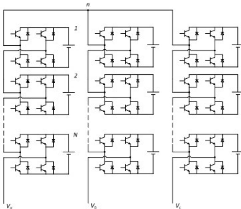
Fig. 7 Topology of cascaded H-bridge inverter
