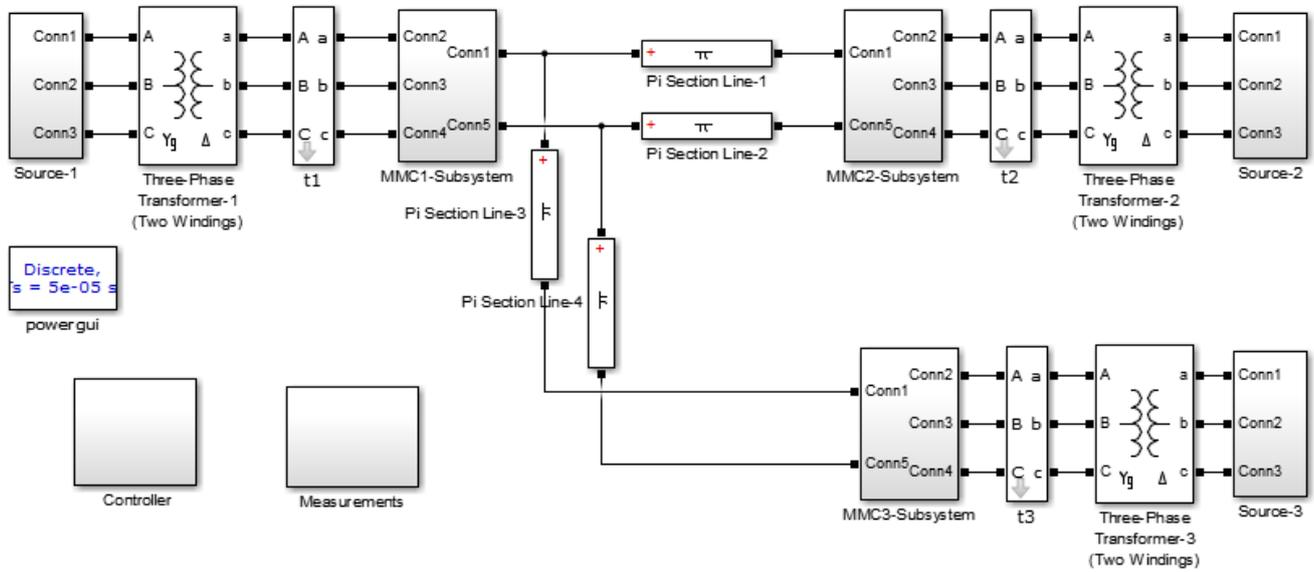
Fig. 13 Simulation diagram of three terminals MMC
