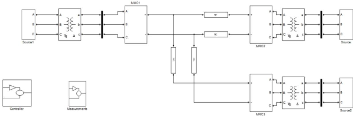
Fig. 9 Simulation diagram of single terminal MMC
