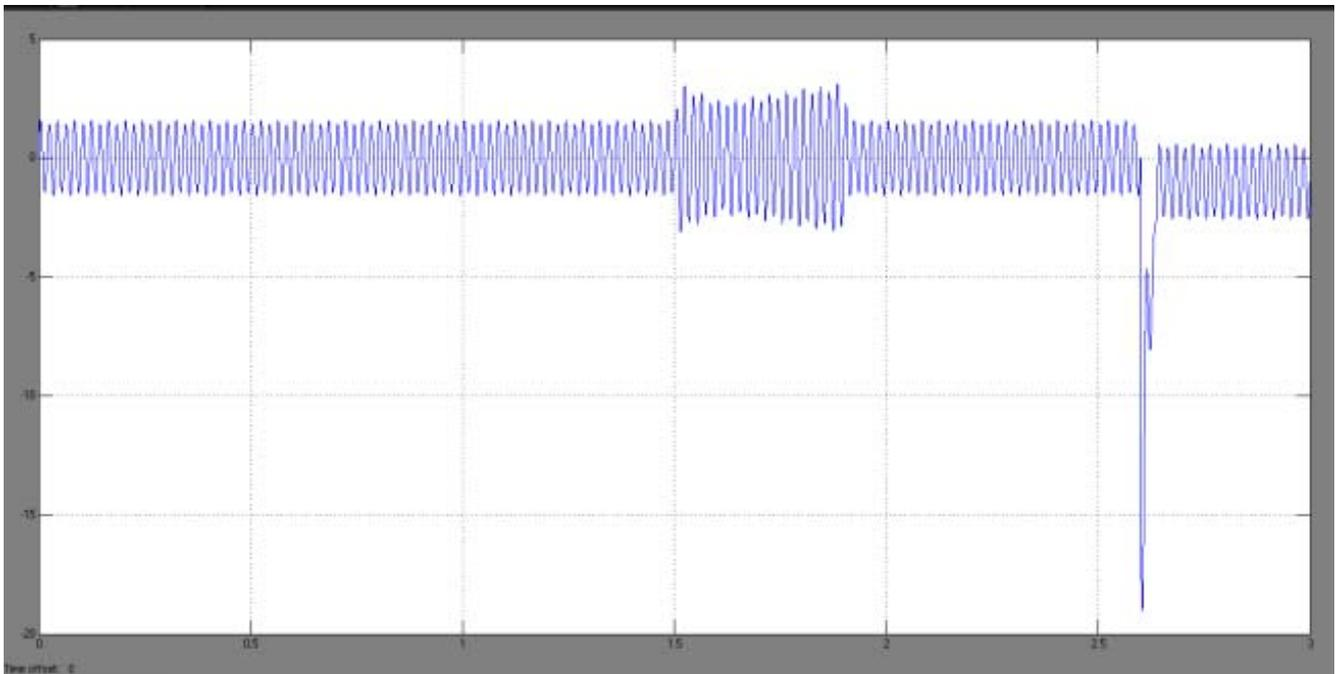
Fig. 18 Waveform of top limb current in phase-A
