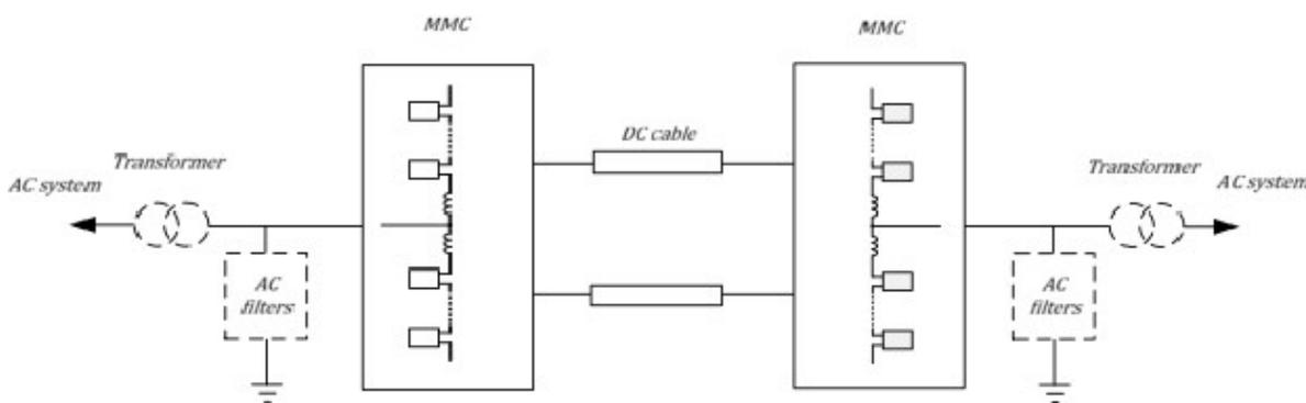
Fig. 5 MMC with HVDC system configuration
