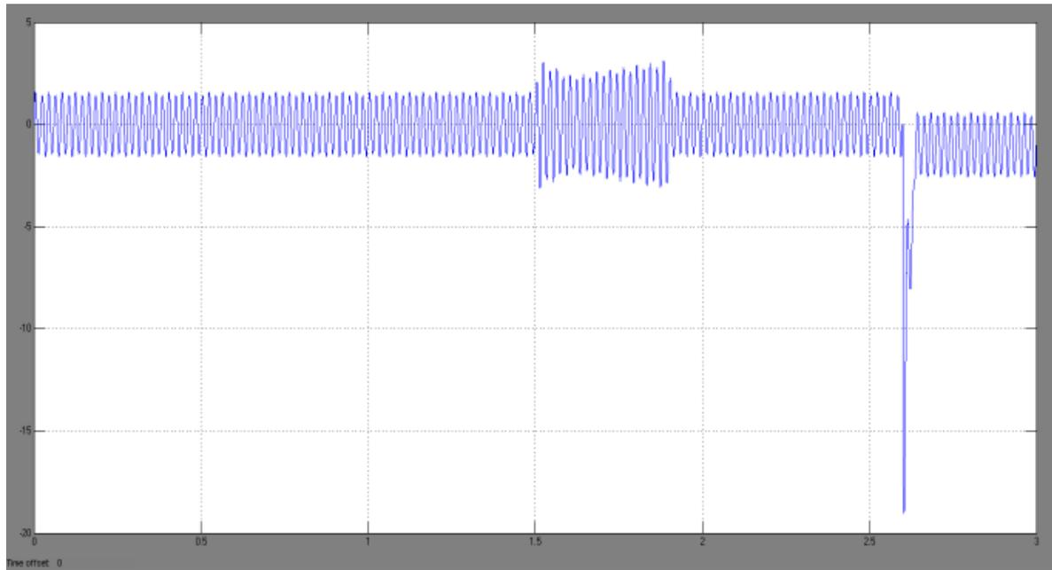
Fig. 15 Waveform of top limb current in phase-A
