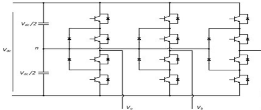
Fig. 6 Topology of three levels NPC converter
