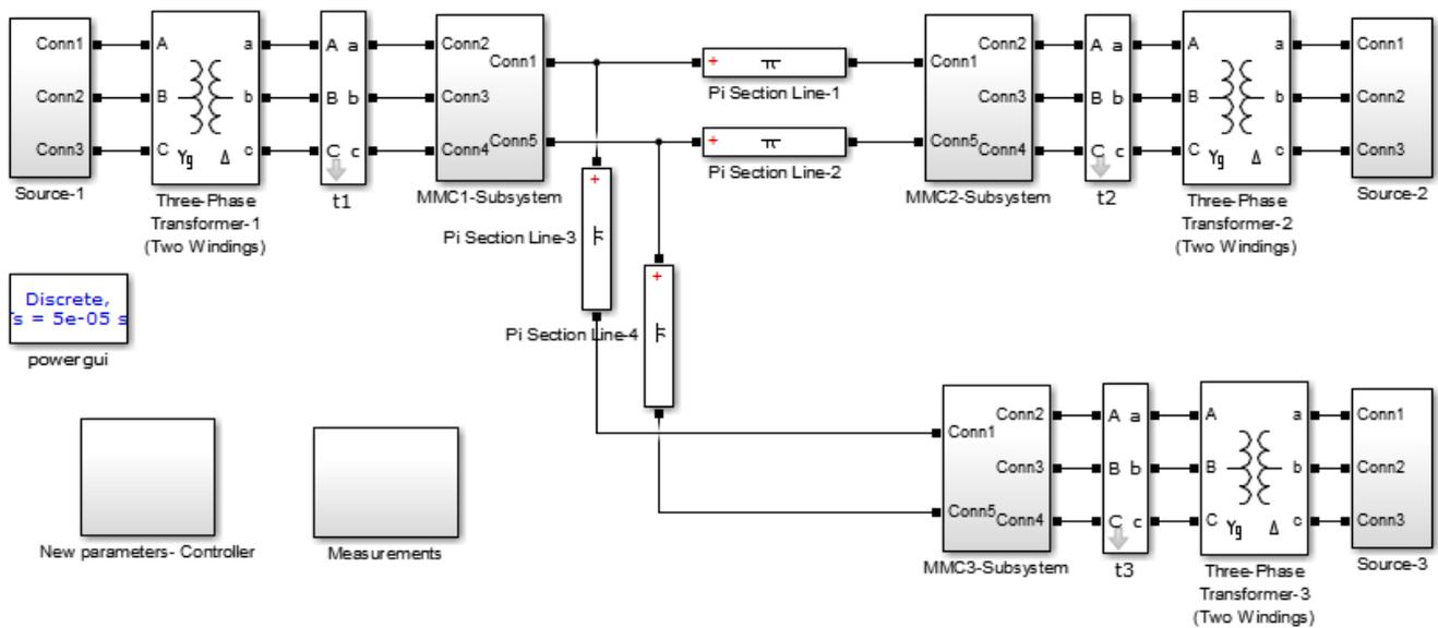
Fig. 16 Simulation diagram of single terminal MMC system with new parameter
