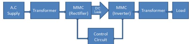
Fig. 1 Block diagram of HVDC system with MMC
