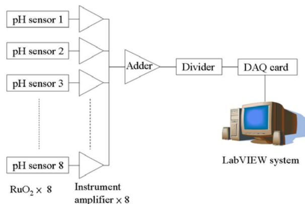
Fig. 1 Schematic diagram of pH array sensing system
