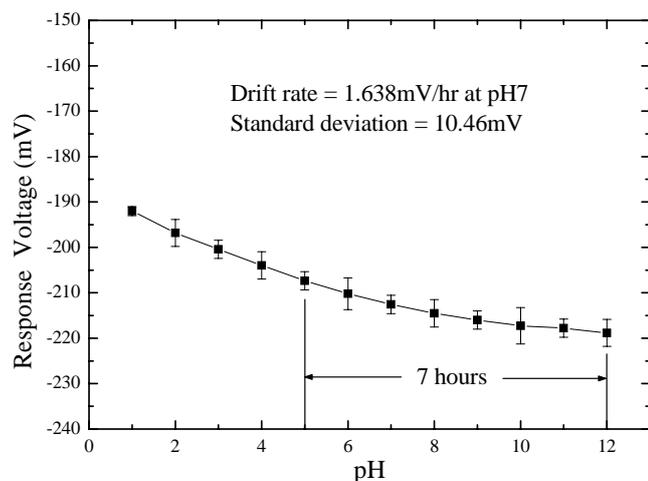
Fig. 3 Drift rate of RuO<sub>2</sub> array sensors in pH7 buffer solution
