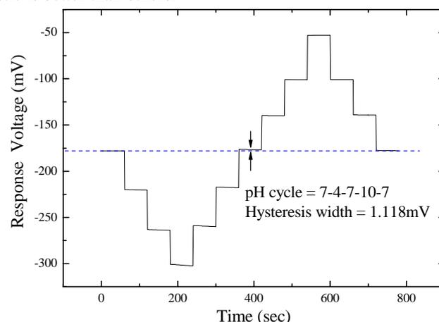
Fig. 4 Hysteresis width of RuO<sub>2</sub> array sensors with pH 7-4-7-10-7 loop cycle
