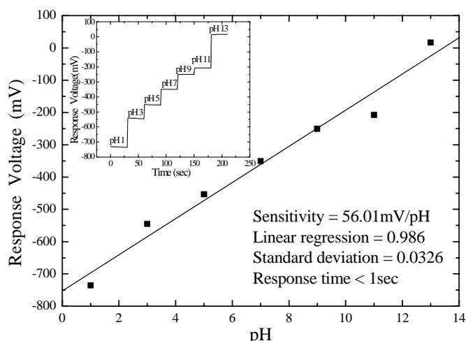
Fig. 2 Sensitivity of RuO<sub>2</sub> array sensors at 25°C
